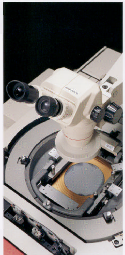
An SZ microscope mounted onto a prober (photo courtesy of Tokyo Electron Ltd.)
