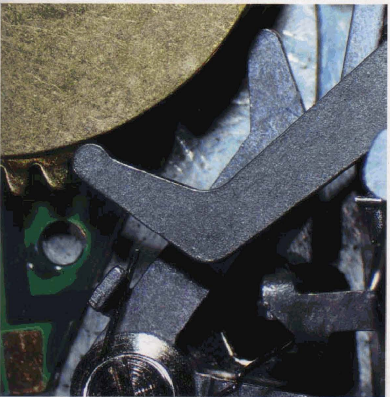
Shutter mechanism for a SLR camera / Incident light illumination
